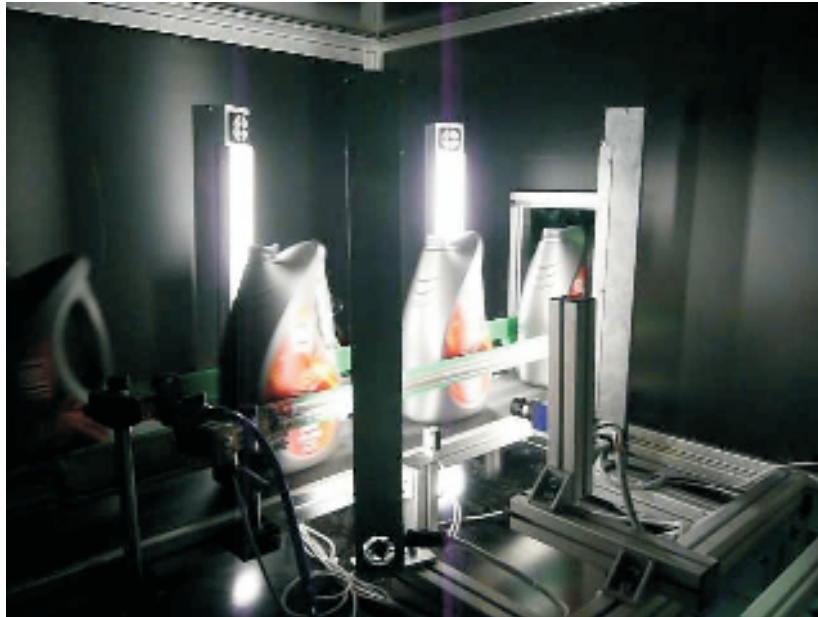
OCR Code reading on plastic bottles
